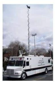
**DEM-10** is a mobile communications vehicle on an ambulance chassis with amateur, public safety and commercial radios.
